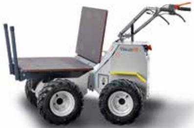
On-board **Smart Battery Charger** with power cable storage (110V / 230V). The TRUXTA electric has a **regenerative-braking system** to help the slow down when stopping; this generates power into battery pack, to increase efficiency and range. **Now with electronic brake over-ride.**
