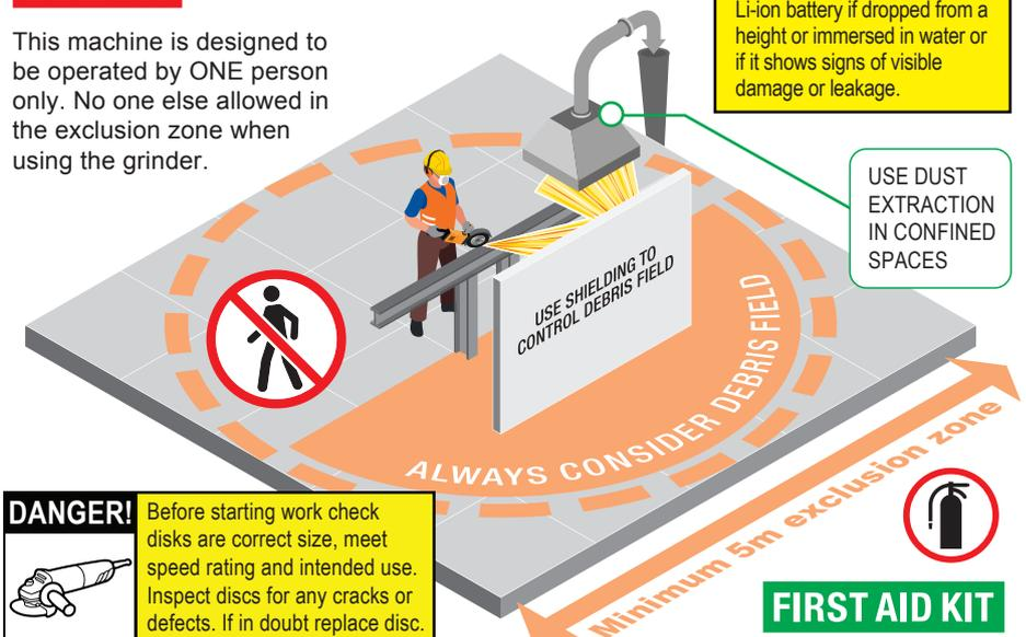
**DANGER!** Before starting work check disks are correct size, meet speed rating and intended use. Inspect discs for any cracks or defects. If in doubt replace disc.
